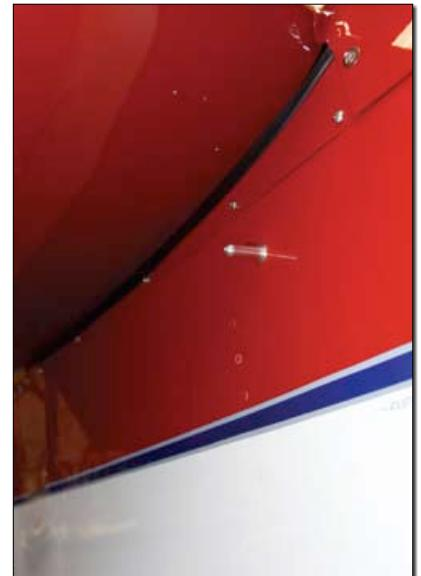
Placing the OAT probe high on the tail cone under the horizontal stabilizer should keep it out of the airstream heated by the engine and exhaust.
