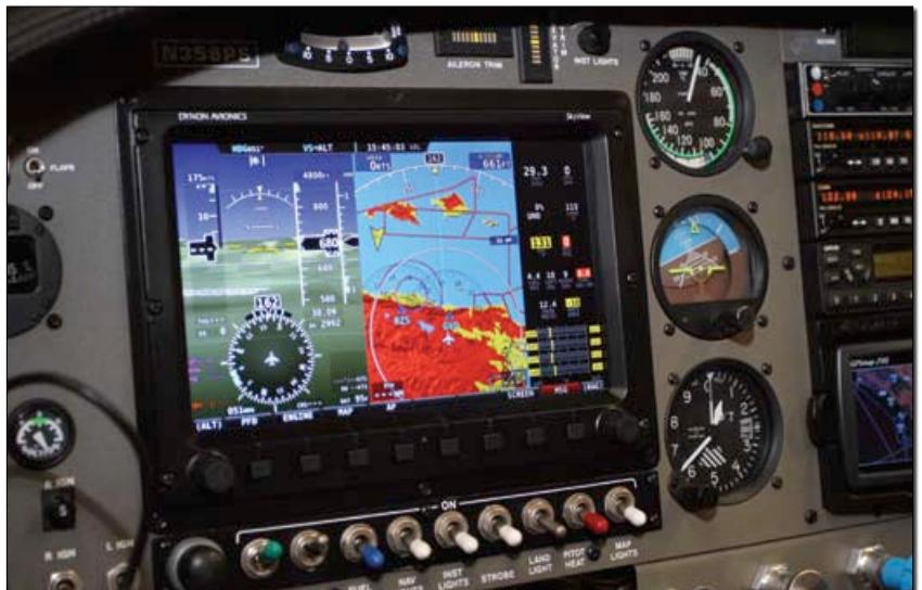
For this single-screen system, the main flight display, moving map and engine strip share space.
