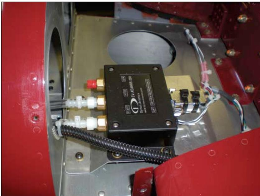
A combined AHRS and magnetometer module forces the location to a magnetically benign portion of the airframe; this is just below the vertical stabilizer fairing.
