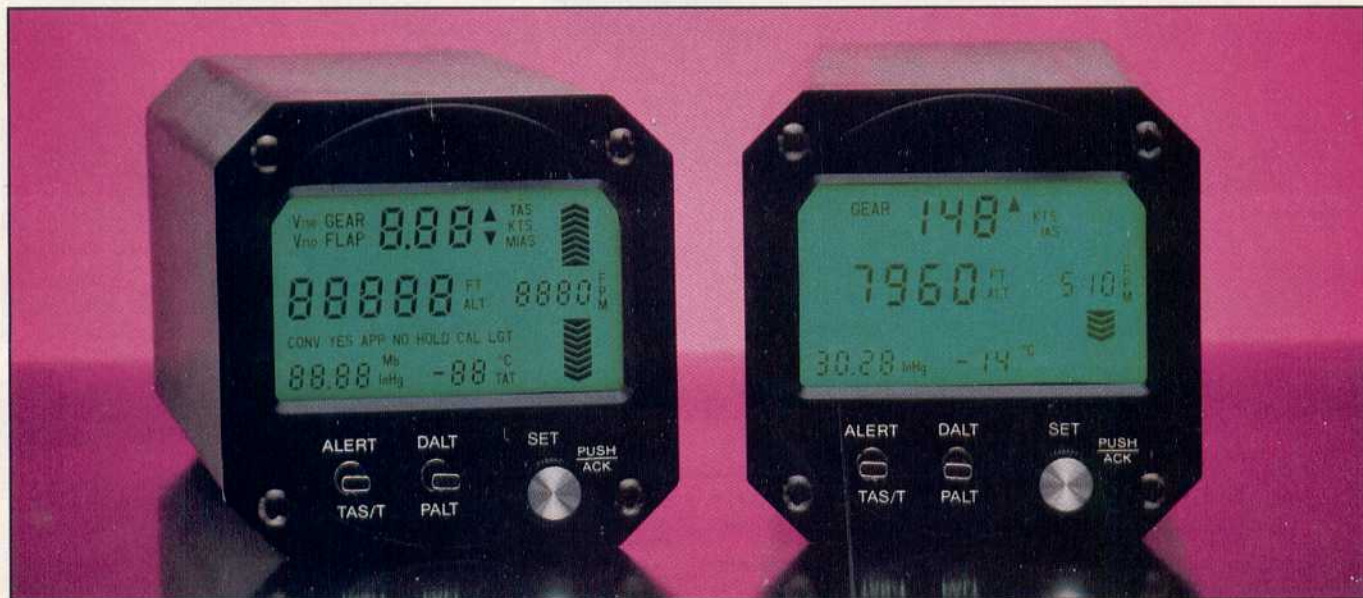
Figure 3. Rocky Mountain Instrument's Micro-Encoder compresses many displays and functions into one unit.
