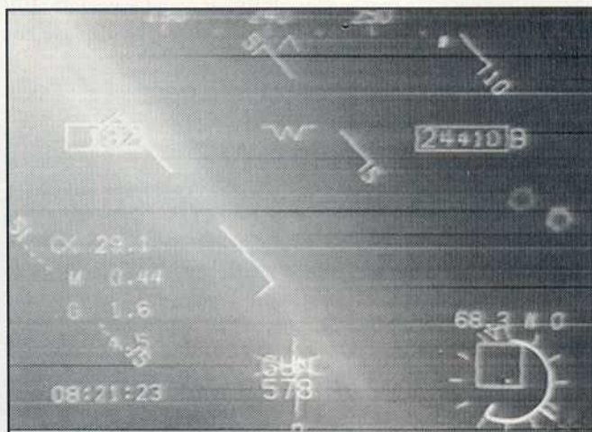
Figure 5. The target aircraft is in the lower part of the target box, beneath the gunsight pipper. Of course, civilian HUDs would not have a gunsight. Where's the velocity vector? It is well below the HUD field of view because the aircraft's angle of attack is 29.1°.
