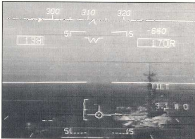
Figure 2. The velocity vector literally shows the pilot where the aircraft is going. Here, the velocity vector is placed beyond the intended point of landing because the landing area is moving!
