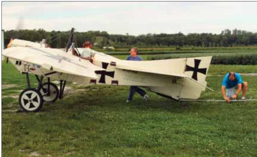
Pull-testing the Taube with its Valley Engineering 2276cc engine, 2:1 PSRU and monstrous 96x60 prop. Mark's doing the reading, and Dick Lemons is watching Tom's thumb for the "Turn her loose" signal.
