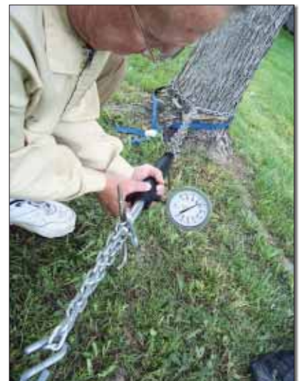
Using a pull-tester with a vertical face gauge makes life easier.
