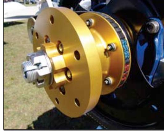
This one-piece propeller hub is another one of Wynne's specialty products designed to put a Corvaire in the air. Making a Corvaire engine flight ready requires a complete rebuild from the crankshaft out and many new parts, but it is still much more affordable than a new or even used O-200 or O-235.
