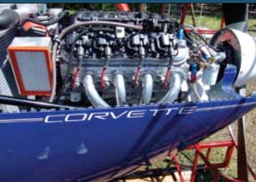
Looking right at home in the nose of an RV-10, Bud Warren's (*GearedDrives.com*) Corvette LS-1 V8 conversion drew crowds at Sun 'n Fun from the moment it was started. Warren says the rear-mounted radiator system has eliminated cooling issues typical with large-displacement engines.
