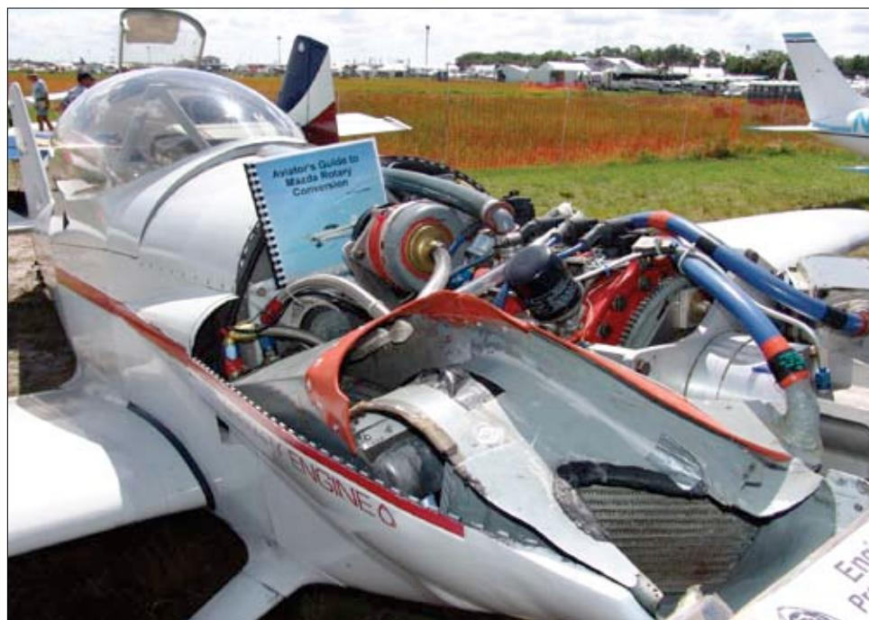
Tracy Crook’s RV-4 may not be the prettiest of the Mazda Rotary conversions, but this flying test bed has logged over 1600 flight hours in Crook’s endless pursuit of perfecting the art of rotary-powered flight.
