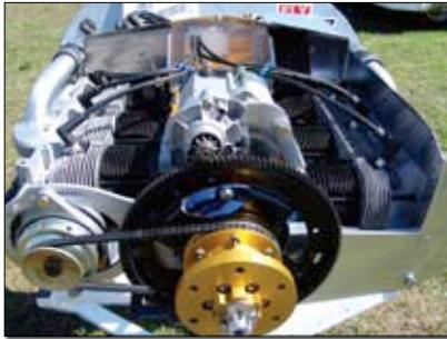
With six horizontally opposed, air cooled cylinders, the Corvaire already has many things in common with traditional aircraft engines. With a displacement of 164 cubics inches, this engine typically produces between 100 and 110 horsepower when converted for aviation use. Can you say LSA?
