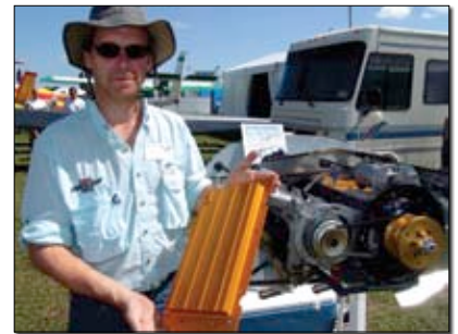
Wynne shows off the current CNC produced, gold-anodized, deep-sump oil pan for the Corvair. It increases total oil capacity to 7 quarts and provides superior cooling over the original 5 quart automotive versions. It's pretty, too.
