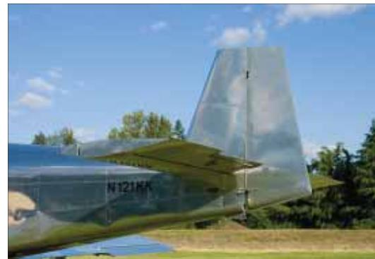
The elevators are mass-balanced, but the simple rudder is not.
