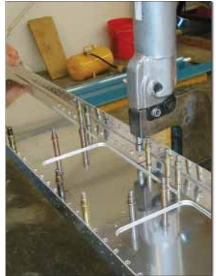
Nothing wrong with power tools! The builders used a large pneumatic squeezer to set the big rivets in the spar.
