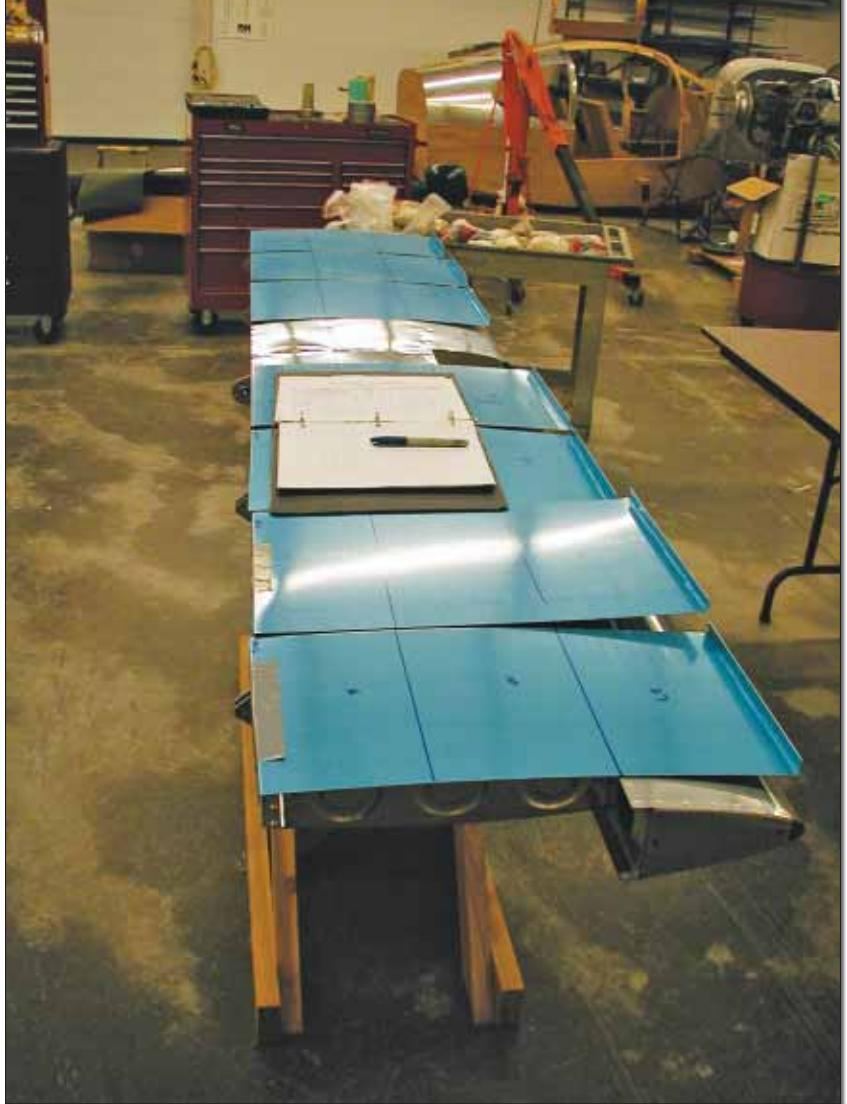
The horizontal stab "test article" is prepared for load testing. Thin sheets of aluminum spread the effect of the lead shot bags.
