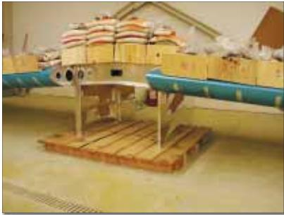
A wing and fuselage center section under test. It takes a lot of lead (and a few lead lackeys) to run this test.
