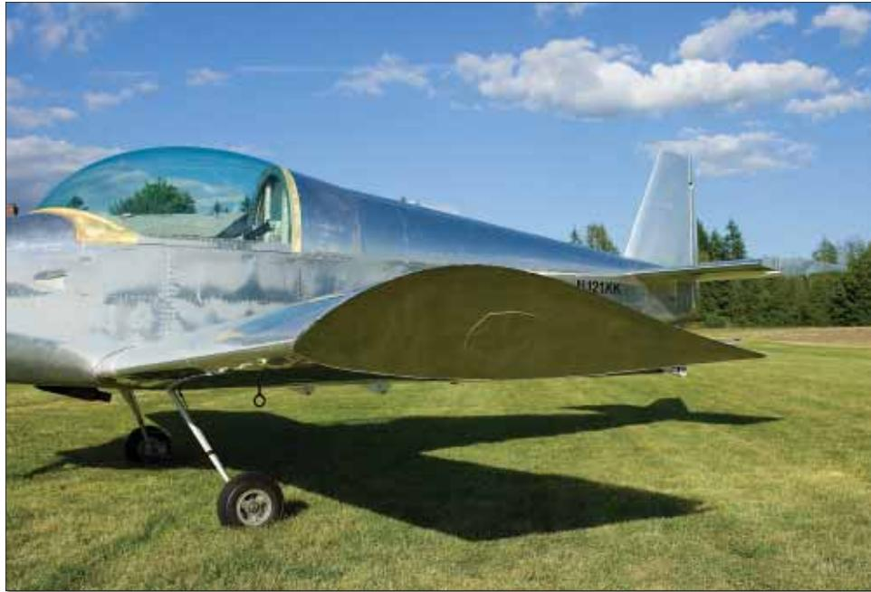
There are all kinds of expensive and complex wingtips out there. This one cost about four bucks, weighs a pound and half and installed in an hour. The plate covers the hole needed to install the aileron pushrod.
