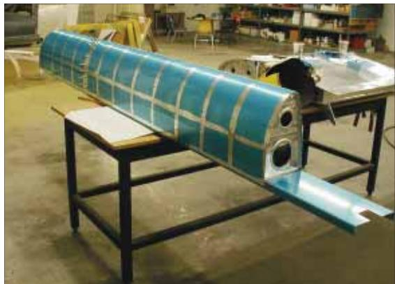
The leading edge of the left wing, mated to the spar.
