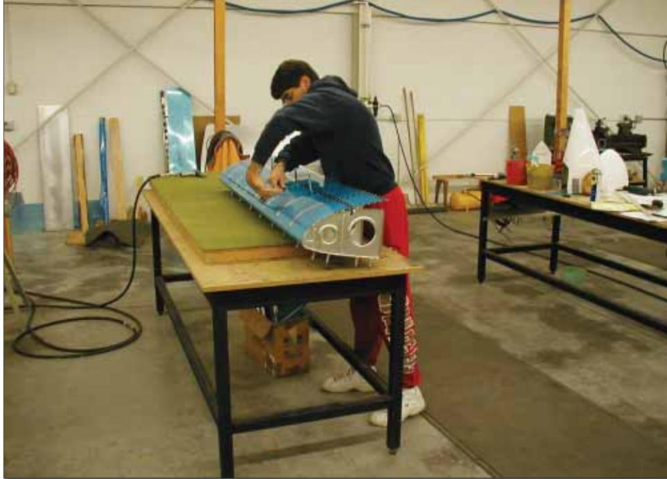
Wing tests completed, the builders started on the leading edges of the flight article.
