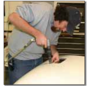
Brian tries his hand at countersinking fiberglass, a tricky prospect any time. Next came nutplates. "How many are there on a Sportsman, anyway?"
