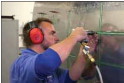
We're riveting now! Blue shirt means Day 3, and the wing is nearly complete, structurally. Some systems remain to be installed.
