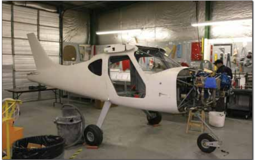
Jumping ahead just a bit. This is the end of Day 5. The airplane is on the gear—has been for a day and a half—and has the engine hung. We pushed the engine hanging ahead in time to be sure the four-into-one exhaust would fit. Yet another prototype part on N30KP!
