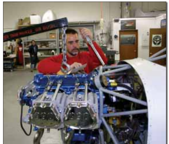
The mighty Barrett IO-390 is hung onto the airframe in the early afternoon of Day 5. Still the first week. Don't get weepy; there's still a huge amount of work left to do.
