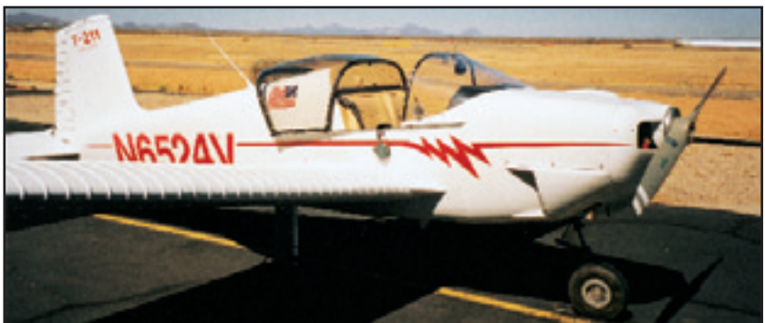
The prototype features corrugated wings and control surfaces for high strength to weight.
