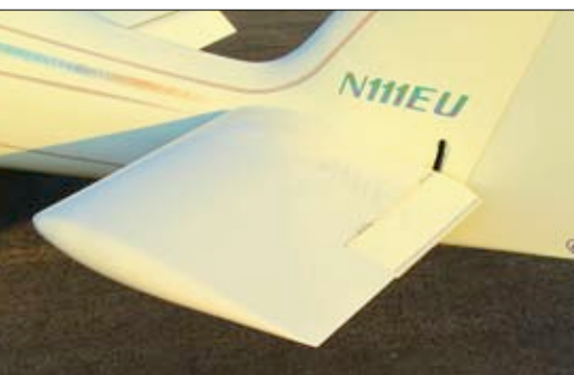
The Europa's generous tail area improves stability. Unusual for a homebuilt, it uses an all-flying stabilator with an anti-servo/trimtab inboard.
