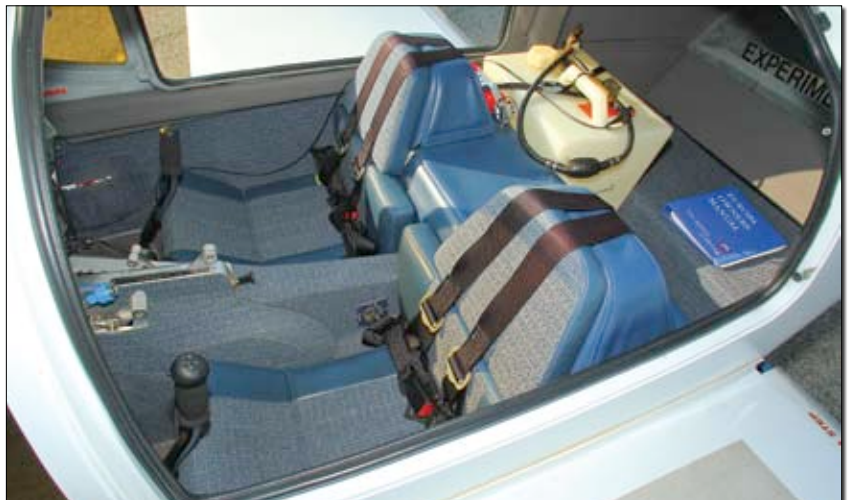
The passengers sit ahead of the mainspar carry-through structure. The tank behind the passenger is the 10-gallon auxiliary fuel supply, supplementing the 20-gallon main fuel tank buried in the fuselage.
