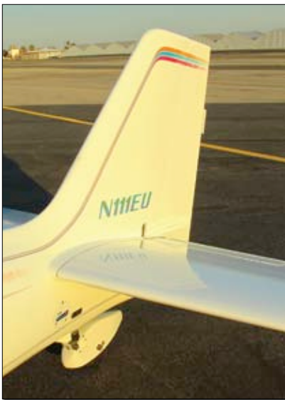
The Europa's generous tail area improves stability. Unusual for a homebuilt, it uses an all-flying stabilator with an anti-servo/trimtab inboard.
