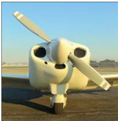
A Rotax 912 and a Whirl Wind prop combine to offer 140-knot cruise speeds in the Europa monowheel.
