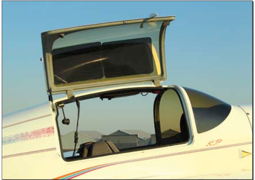
Large gullwing doors permit easy access to the cabin and allow you to reach the baggage compartment without too much stretching.
