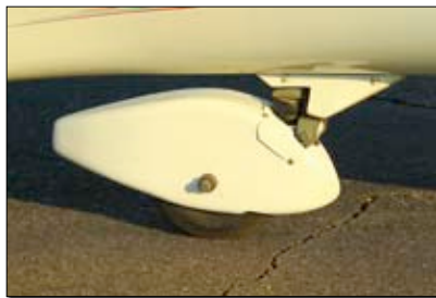
The single beefy main tire is kept at a relatively low inflation pressure to reduce landing shock. The faired tailwheel is under the empennage; later Europas have the tailwheel further aft.
