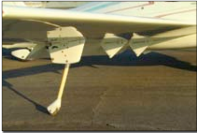
Outriggers balance the airplane on the ground and retract aft when the gear/flaps are raised.
