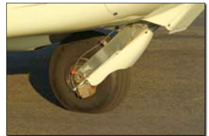
The single beefy main tire is kept at a relatively low inflation pressure to reduce landing shock. The faired tailwheel is under the empennage; later Europas have the tailwheel further aft.
