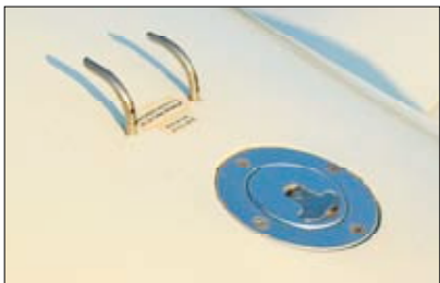
The fuel filler is behind the cabin along the roofline. Fuel vents face forward.
