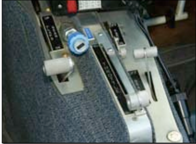
Handles galore. The large metal lever to the left extends the flaps and the single landing gear together. The throttle is in the center, with the single brake to the right.
