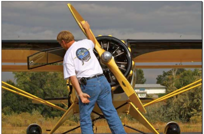
Part of the cold-start ritual is to rotate the prop by hand to ensure the lower cylinders have not filled with oil. Yes, just like the big radials.
