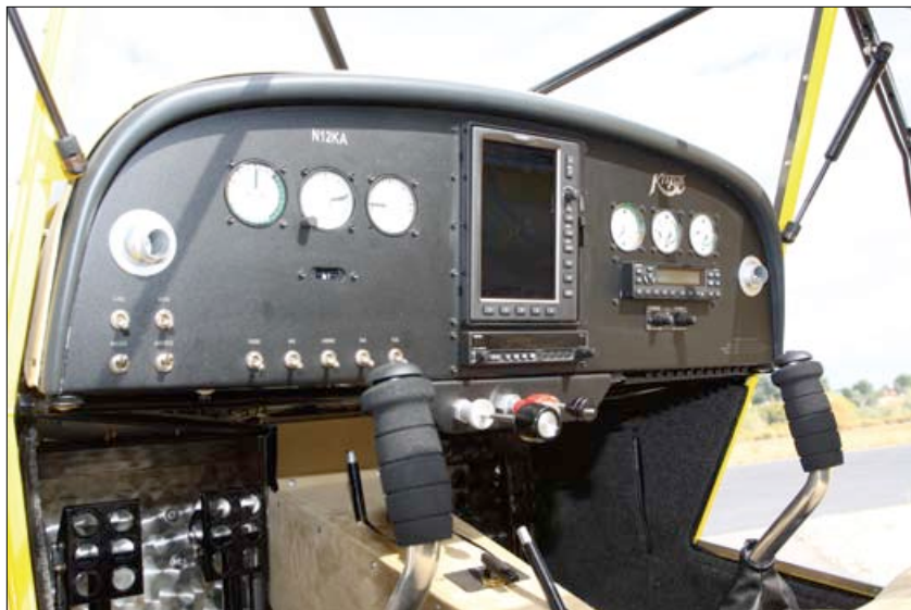
Kitfox owner John McBean almost said “no glass,” but couldn’t resist the Garmin GPSMAP 696 moving map. The rest, alas, is pretty basic.
