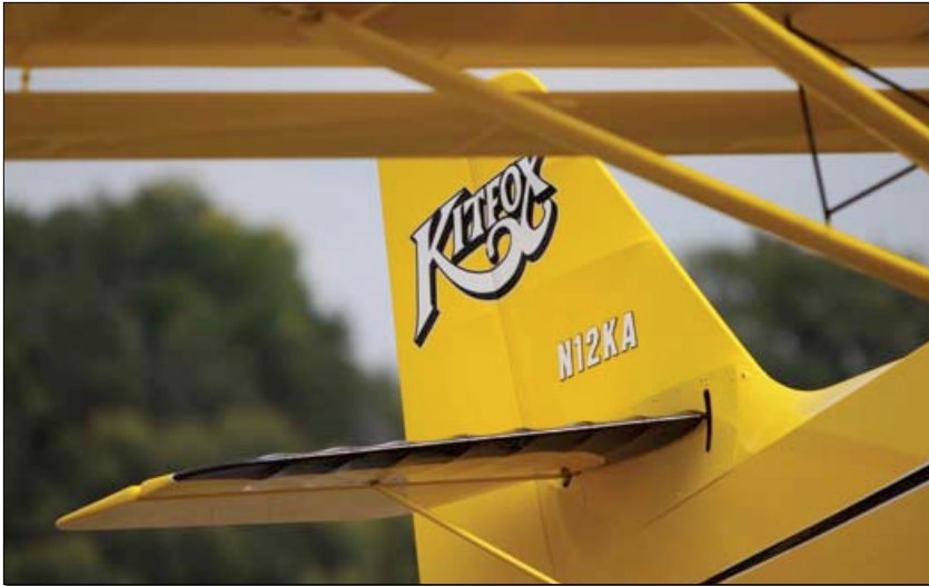
An airfoil-shaped horizontal stabilizer is optional—as opposed to a simple flat surface. It improves low-speed response.
