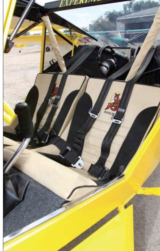
Comfortable sling seats offer reasonable room for large occupants. The seats don’t adjust, but the rudder pedals do.
