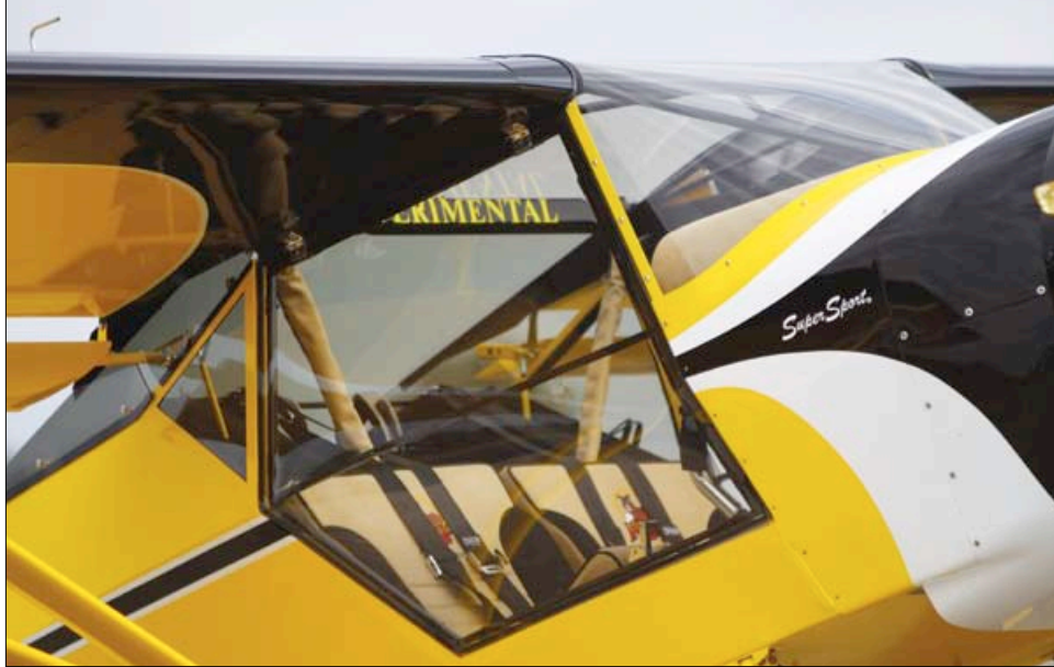
Lexan doors combine with a full overhead glass panel to provide exceptional in-flight visibility.
