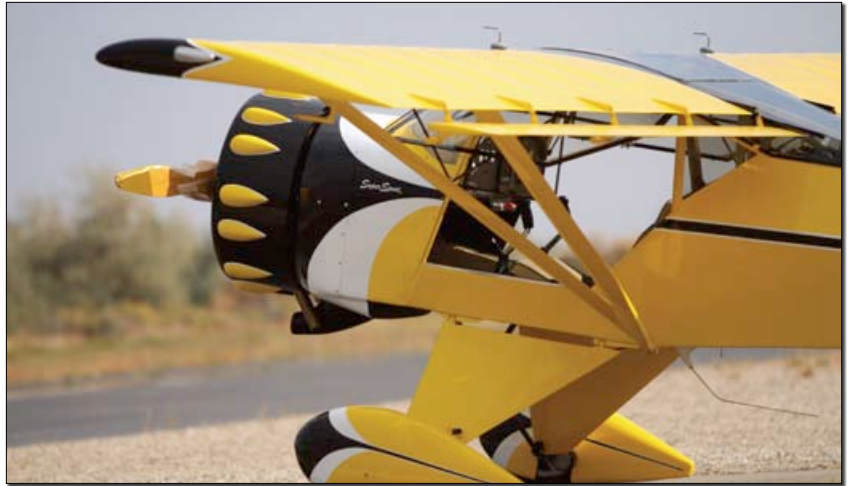
Flaperons continue to be a Kitfox design hallmark. They move individually for roll and extend together for flap effect.
