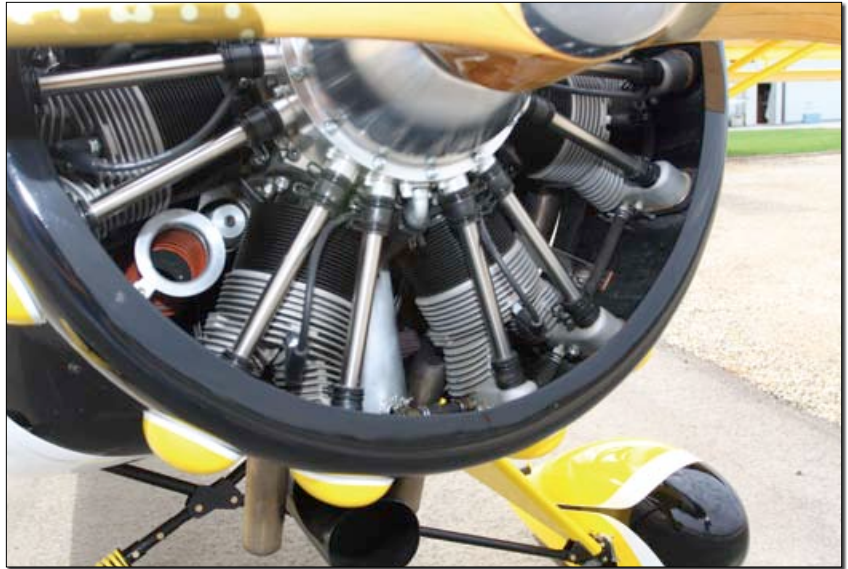
It's a tidy installation of a nicely finished but generally conventional (if quite small) air-cooled radial.
