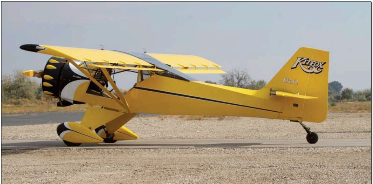
Looks bigger than a regular-edition Kitfox, doesn’t it? Well, it’s not. Aside from the new gear, the airframe is identical to the other Super Sports from the firewall aft.
