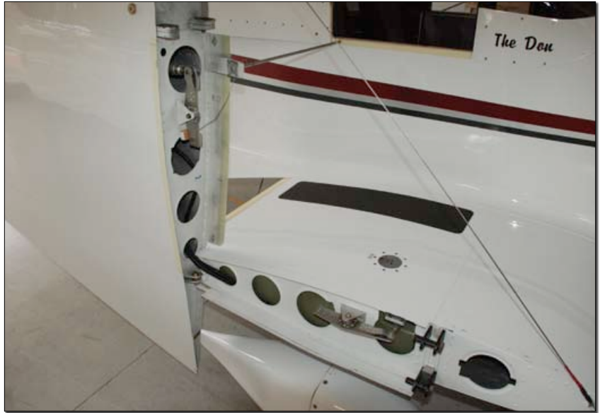
No aileron hookup is required because the center walking beam can always push against its outer counterpart. The inboard wing fuel tank filler is located here.
