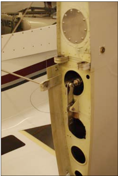
Here you can see the access plate for the outboard fuel tank in the wing leading edge, and that tank's fuel drain.
