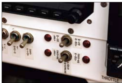
Fuel management is not done with valves; it's done by pumping fuel into the 25-gallon fuselage tank from wing tanks. Two switches control four pumps.
