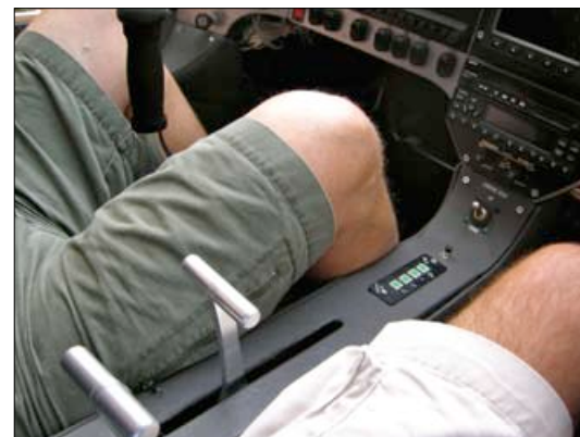
From the left (aft): throttle, wheel brake, flap pre-select and gear. A voice reminds you to think about whether you're configured for water or land.
