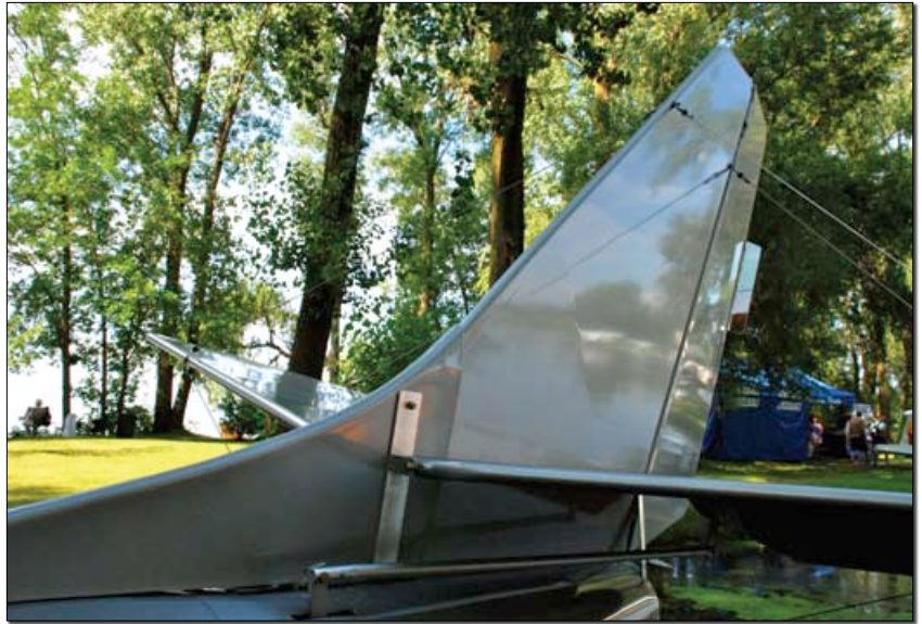
Shades of the old F-101, the new horizontal tail is 25% larger, and has dihedral to help keep the tips out of the weeds.
