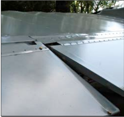
Gap and aileron seals increase cruise speed. For slow aircraft, every little bit helps!
