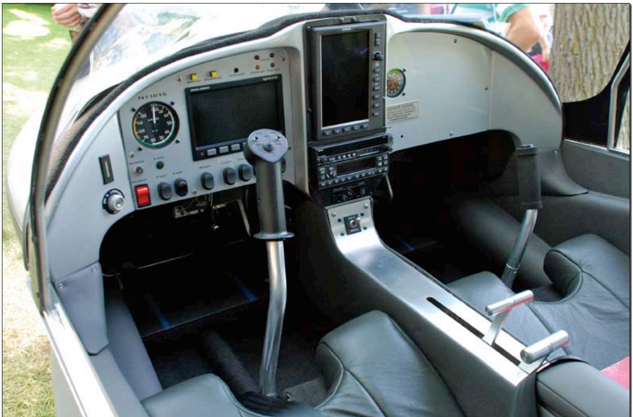
The cockpit. Note the analog airspeed indicator, easy to read in just a flash. In the center console, the two T-handles are the brake (forward) and the throttle (aft).
