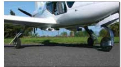
The Orion’s tricycle retractable landing gear is all composite and immensely strong.
