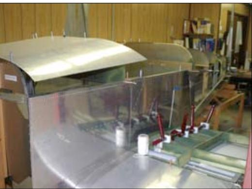
This is a kit project under construction by local builders in borrowed space at the Mustang Aeronautics factory. Pre-built wings saved considerable construction time, and the pre-dilled fuselage bulkheads provided pilot holes for attaching the fuselage skins.
