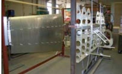
By purchasing either fully built or partially built wing options, the Mustang kit builder doesn't need to acquire his own wing jig and gets into the air with a lot fewer rivets to drive.
