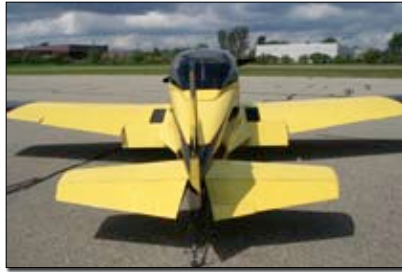
The Mustang II's generous tail feathers provide good handling and stability for cross-country travel.
