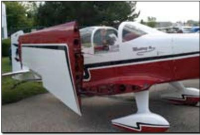
With the wings neatly folded, requiring only a few minutes of work, Scheltema's Mustang II can be rolled onto its trailer and taken home.
