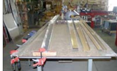
The Mustang wingspars attach to a pre-built center section, with dihedral angle set and critical riveting done.
