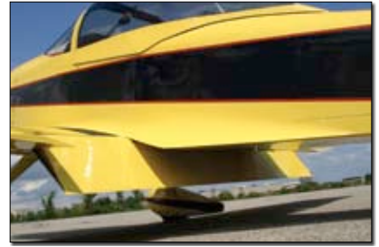
The Mustang II uses a wide manually actuated flap that spans the center section under the fuselage as well as the inner portion of the wing.
