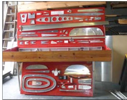
As shown on display for the factory open house, Mustang parts can be purchased in kit form or individually, saving tedious creation of form blocks, bending of flanges, measuring and drilling.
