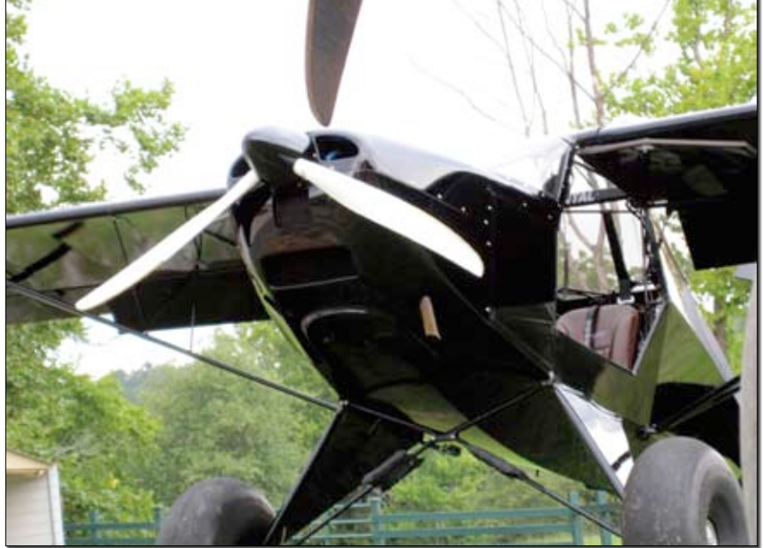
Yes, it is that tall. With the optional bush tires and longer gear legs, the Highlander stands head and shoulders above most other light planes. The bush gear has three weldments on the lower longeron for extra strength.
