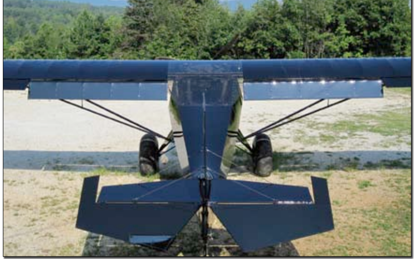
The secret to a mid-20s stall speed is having 40° of flaps and a bucket full of vortex generators. Simple systems and large control surfaces are well matched for the low speeds the Highlander is capable of.
