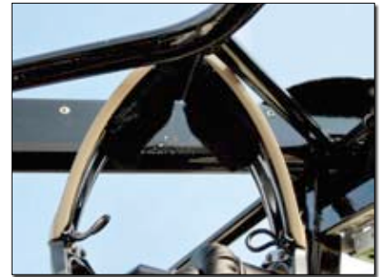
A small hook is part of the structural cage. Purpose? To hang your headset.
