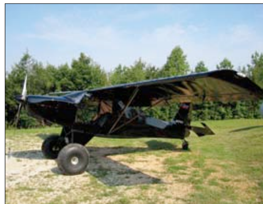
This is the Just Aircraft factory demonstrator with the mighty Rotax 914. With two adults on board, this aircraft can climb at more than 1800 feet per minute.
