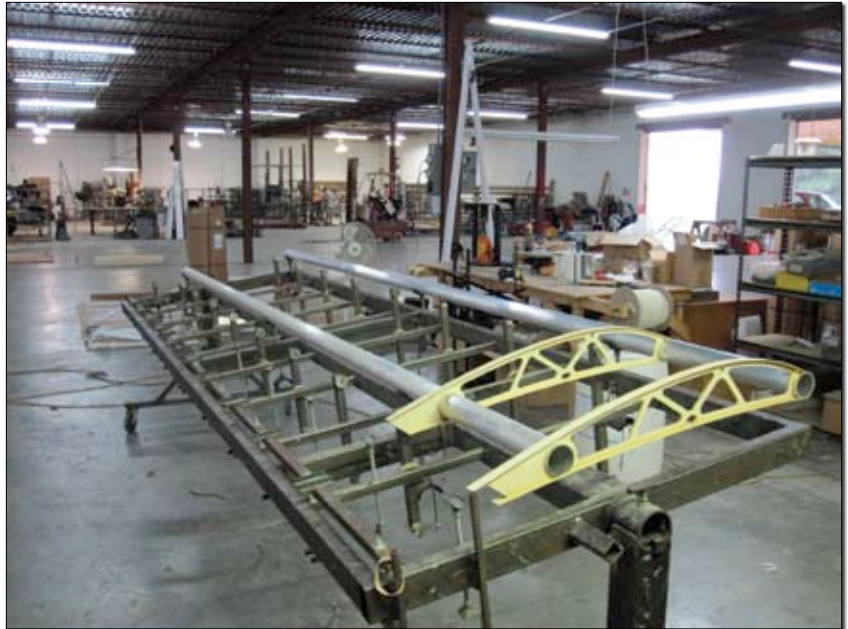
Select the quickbuild wing option and your wings will be assembled in this jig, virtually guaranteeing straight wings. While an option, quickbuild wings are strongly encouraged by the factory.
