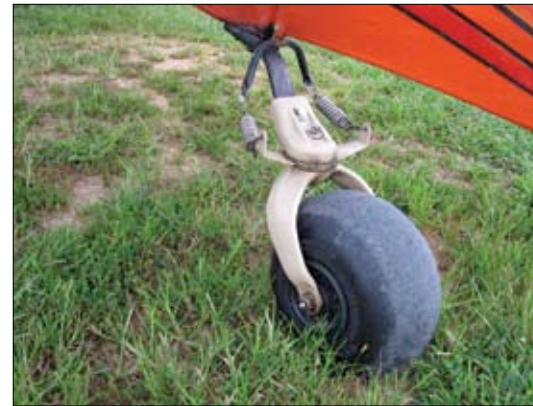
That ain't no dinky rollerskate wheel. At 11 inches, it is much larger than the mainwheels on many homebuilts.
