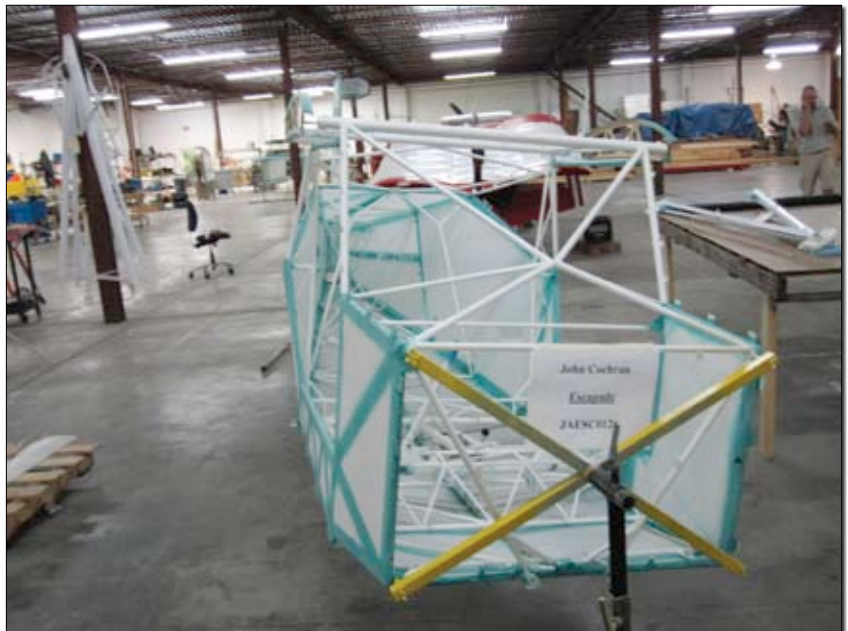
A 4130 steel-tube fuselage cage and lightweight 1.7-ounce polyester fabric contribute to the Highlander's unusually high useful load and safety.
