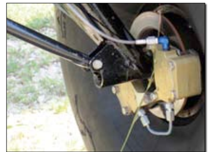
Dual brakes, big tires and weeds—signs of a bush plane. In the Highlander, stopping power combined with a low stall speed make easy work of short-field landings.
