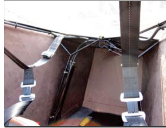
Not only is there a large useful load by LSA standards, there is room for your stuff. The vertical tube is the header tank for the dual wing tanks.
