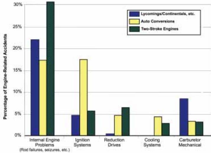
Figure 5: Traditional Engines vs. Auto Conversions & Two-Strokes
