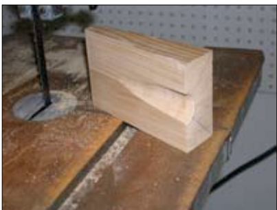
Cut along the angle with a bandsaw or sharp handsaw. When the block falls open, there's a conical recess that is the female side of the die.
