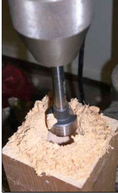
A 1-inch Forstner bit cuts into the endgrain of a block of straight-grain fir.
