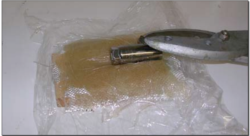
The female die, appropriately waxed, can also be used to form a fiberglass fairing.
