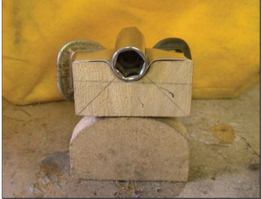
A piece of water pipe of the same size as this deep socket may be used as the male die.
