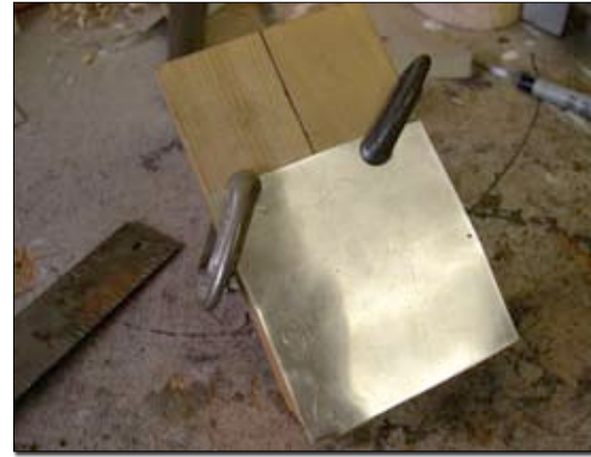
A piece of dead soft aluminum will form the fairing. The process starts by tightly clamping it across the hardwood "cone." Changing the angle of the block will change the shape of the cone.
