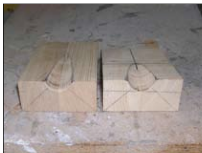
Cut along the angle with a bandsaw or sharp handsaw. When the block falls open, there's a conical recess that is the female side of the die.
