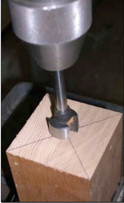
A 1-inch Forstner bit cuts into the endgrain of a block of straight-grain fir.
