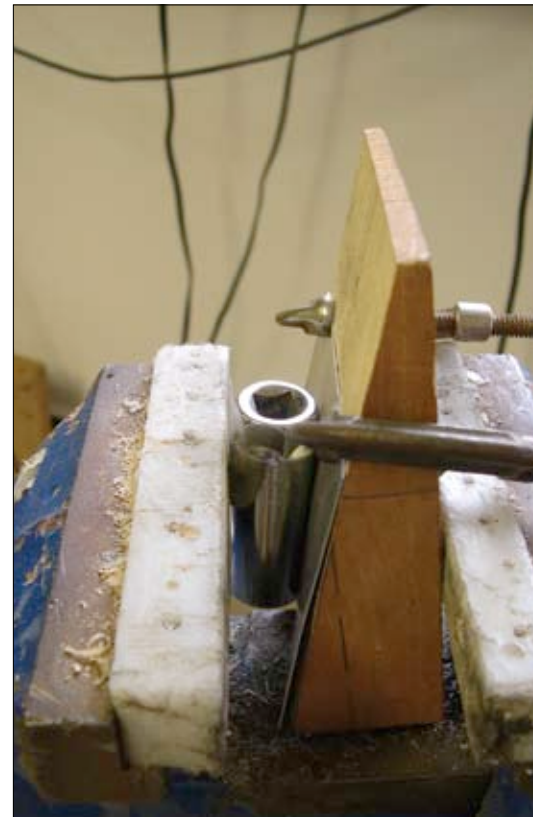
A vice supplies the power to force the dies together and form the aluminum.
