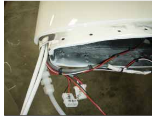
Electricity for the leading-edge panels is taking up the D-section void.
