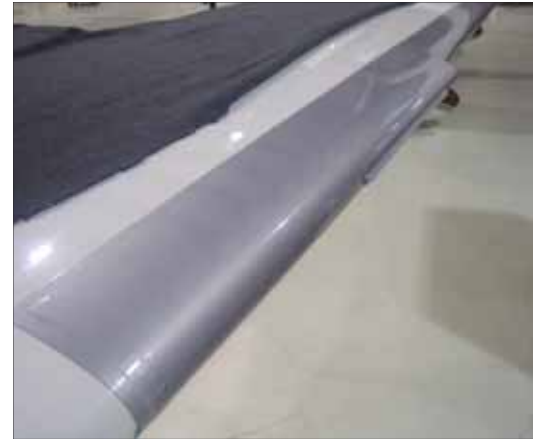
Each Therm-X panel has different element circuits divided into parting zones and shedding zones. Plus, not all panels are powered simultaneously, reducing peak current requirements.
