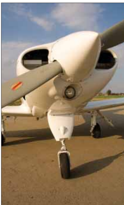
That's a Lycoming IO-320 under the cowling. If you want the 180-hp 360, be prepared for blisters on the upper cowling.
