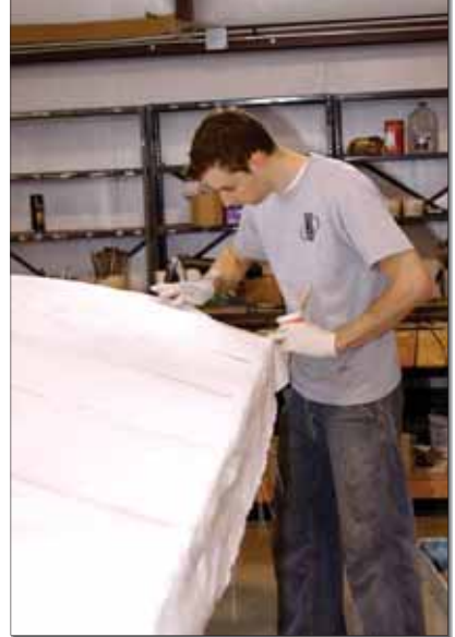
Work in the Homedale, Idaho, factory continues on the next SLSA to be built. Kitfox uses the PolyFiber fabric and finishing system.
