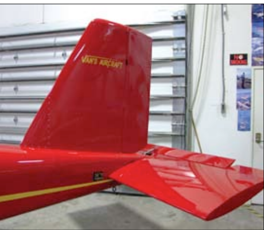
Designing the RV-12 for economical take-home capability led to using a stabilator.
